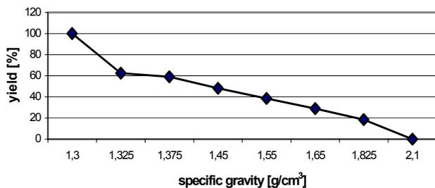
Figure 4. Coal enrichment curve given by Gauss kernel function application
