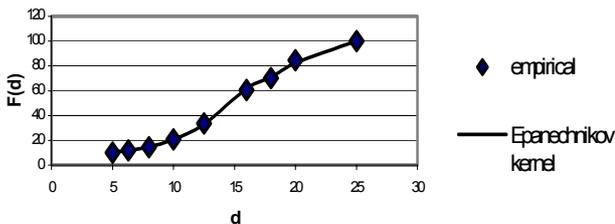
Figure 1. Distribution function plot given by Epanechnikov kernel (stage I) -  $s_r=1,01$ .
